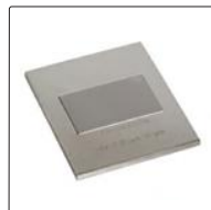
roughness calibration block Ra2.97µm (included)
